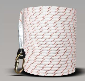
**ERAIDED ROPE ANCHORAGE LINE** Rope ends splices & covered with Polyethylene protective sleeve. Abrasion resistant thimbles provided within loops. One side loop thimble while other side equipped with karabiner GI-SK-01 with an opening of 18 mm. Breaking Strength 25KN.
