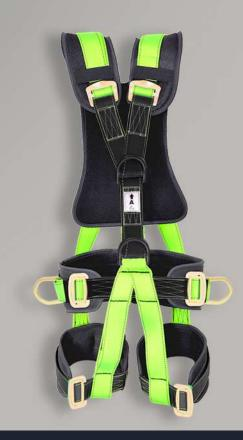
Full body harness made up of 44 mm wide highly UV rays resistant polyester webbing one dorsal D-ring for fall arrest. One chest attachment (sternal) D-ring for fall arrest one ventral D-ring at abdomen for rope access two lateral D-Rings at waist for work positioning adjustable shoulder, thigh straps & waist belt Shoulder straps provides extreme comfort due to comfort padding 2000 gm ± 10 gm.
