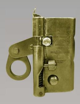
Rope Grab Fall Arrester made of high strength galvanised steel. Working on unique Self Braking System which works on 14mm to 16mm 3 strand twisted rope. Moves along with the user climbing up or down and locks him in the case of a fall. Double Safety Opening System (Equipped with antigravity pin to prevent accidentally locking the fall arrestor in reverse direction)
