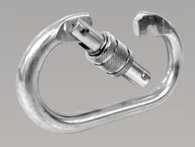
STEEL SCREW Karabiners for fall protection meet EN standards for use as part of a fall protection system. They create a connection between two anchoring points, such as connecting lanyards/self-retracting lifelines (SRLs) to anchors or connecting lanyards to harnesses. These carabiners have a minimum tensile strength of 25KN, and a locking mechanism that prevents the Karabiner from opening on its own
