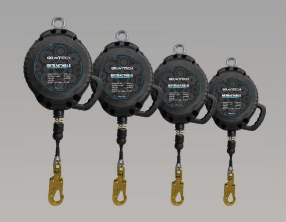
Retractable fall arrester is designed 6mtr. 10mtr. 15mtr. 20mtr. to protect its user from fall arrest. Main feature is to arrest the fall within 2meters and reduce fall forces below 6kN.
