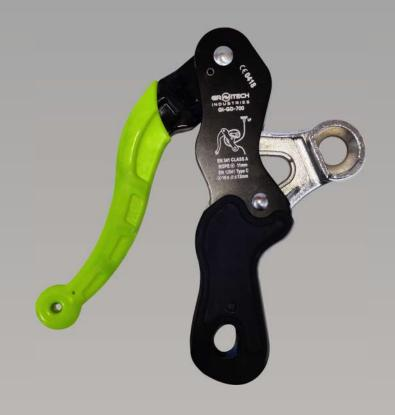
t is equipped with a unique self-braking system that initiates the brake as soon as the handle is released or clasped too tightly. Equipped with polymer-coated cover to protect the user from the heat generated during descent.
